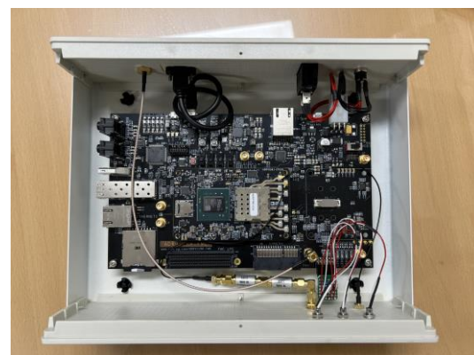
Hardware of FPGA based Rel time GNSS Signal Generator
